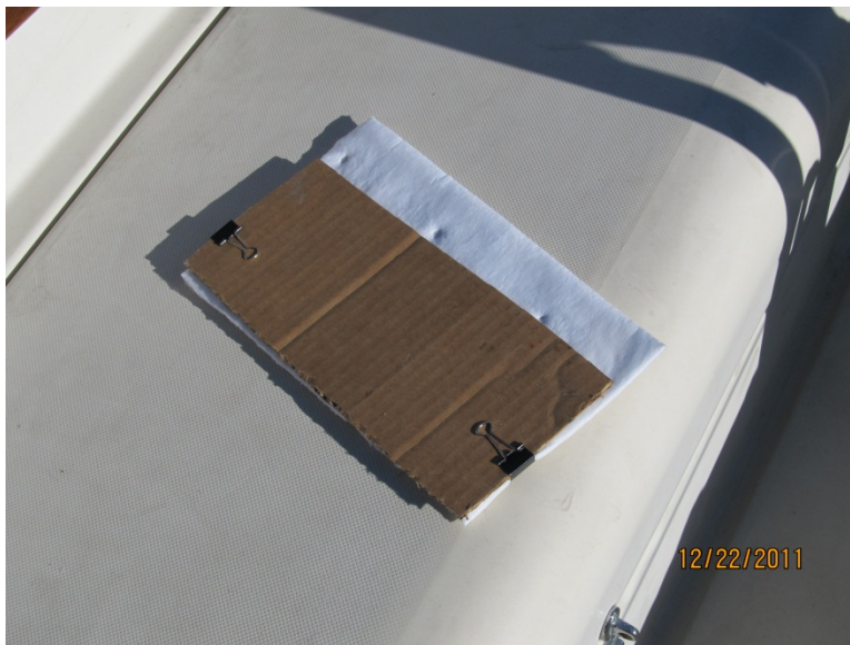
Figure : Details showing how pad is larger than cardboard, allowing it to be folded up underneath filter.
