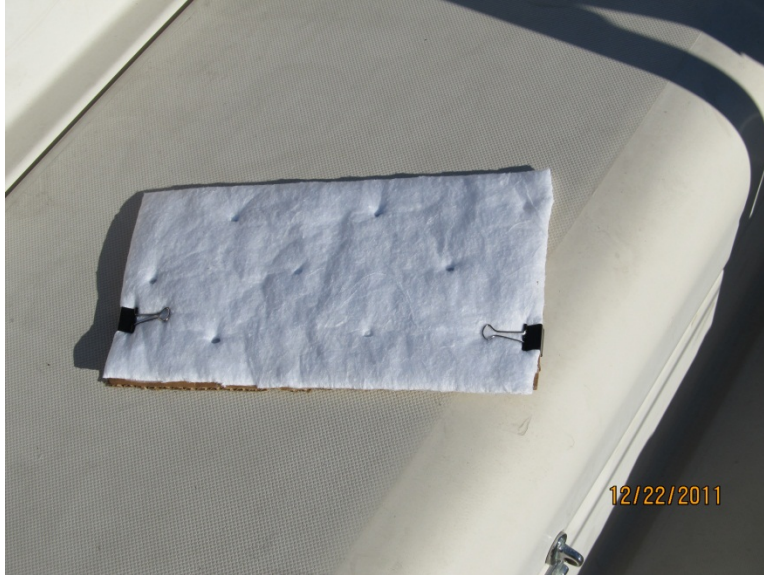
Figure : Oil absorbent pad cut to fit and mounted on cardboard platform with binder clips.
